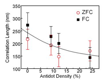
FIG. 7. (Color online) Correlation length of the inverted domains for  $Ni(6 \text{ nm})/\text{FeF}_2(70 \text{ nm})$  as a function of the AD, measured at zero field and 30 K, upon ZFC from 296 K (red) and FC (black; same protocol as in Fig. 6). The dashed line is a guide to the eye.
