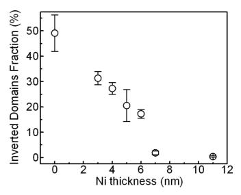
FIG. 4. Fraction of inverted domains for Ni/FeF $_2$ (70 nm) bilayers as a function of Ni thickness, measured at zero field and 30 K, after ZFC from 296 K. The error bars represent the standard deviation of the mean but do not include smaller systematic errors arising from either the PEEM measurements (e.g., due to an inhomogeneous illumination of the XMCD images) or the analysis procedure (caused by image drift correction and evaluation of the area of the domains).
