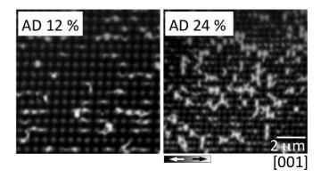
FIG. 5. XMCD images at the Ni edge of the domain structure of square arrays of 200 nm in length square antidots with antidot densities AD=12 and 24% patterned into a Ni(6 nm)/FeF<sub>2</sub>(70 nm) sample, measured at zero field and 30 K after ZFC from 296 K. The arrows indicate the magnetization direction. Note that the gray contrast represents the absence of XMCD signal at the position of the antidots. The scale bar is the same for both images.
